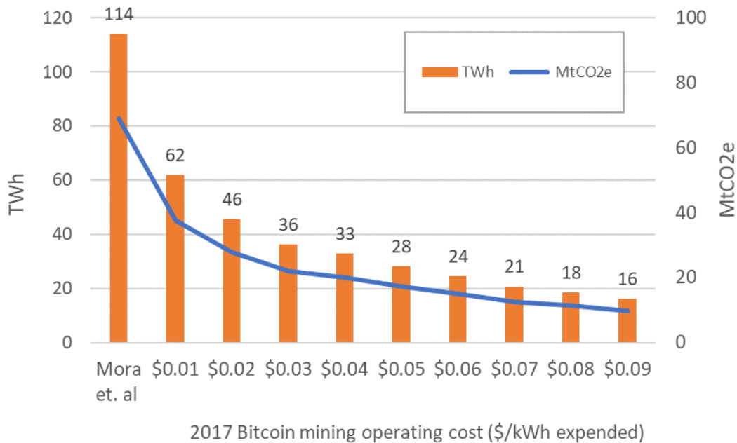
Supplementary Figure 6. Mora et al. model estimates of 2017 Bitcoin electricity use and CO 2 emissions when unprofitable rigs were excluded from their selection pool, at different operating cost assumption levels.
